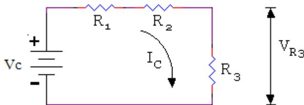
$$R_0 = R_T = R_1 + R_2 + R_3$$
