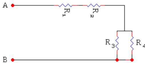
$$R_{ab} = R_1 + R_2 + \frac{1}{\frac{1}{R_3} + \frac{1}{R_4}}$$
