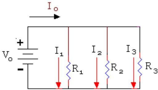
$$R_T = \frac{1}{\frac{1}{R_1} + \frac{1}{R_2} + \frac{1}{R_3}}$$
